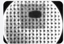
Missing solder ball on standard BGA
